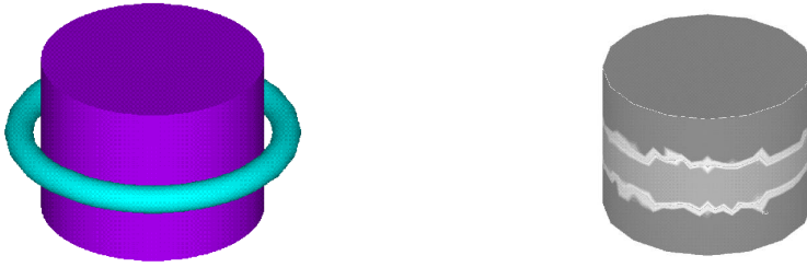
FIG. 2.1. Cylinder-symmetric workpiece with uniform inductor distance and the corresponding distribution of austenite.
